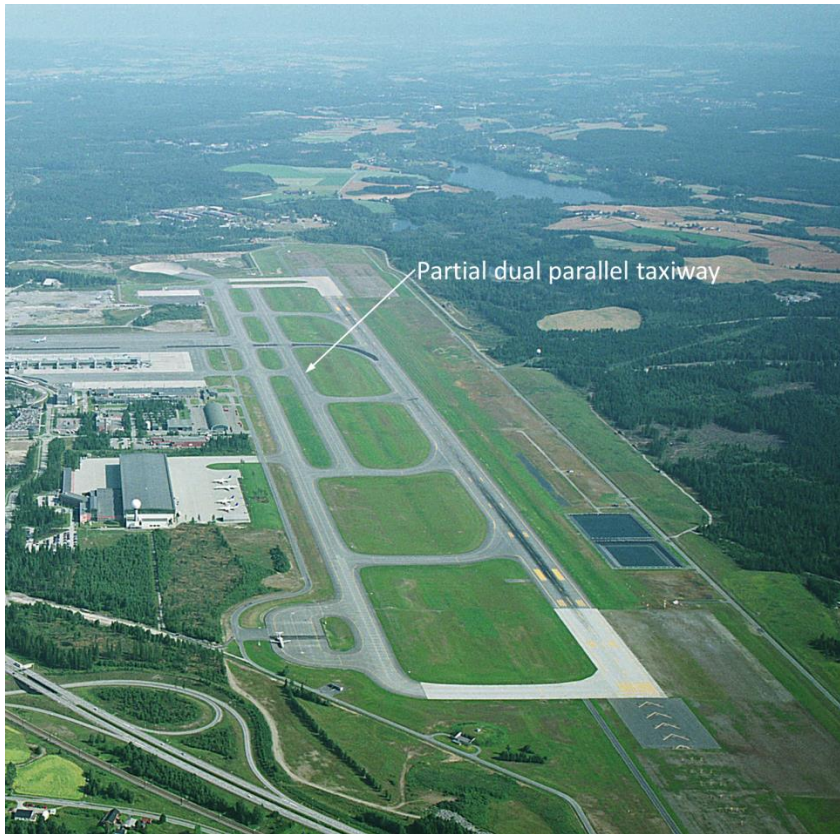
Figure 2: Example of an airport with a partial dual parallel taxiway (Photo: Oslo Lufthavn AS)
